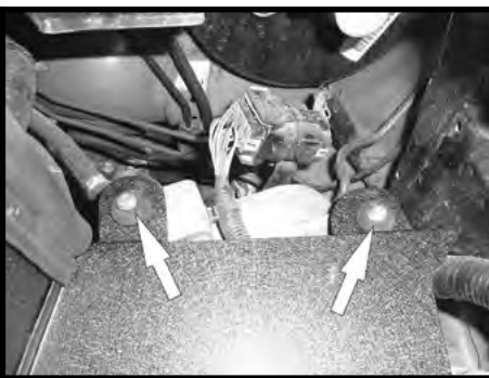
Step 9 Install the heat shield, sliding the fresh air tube into the reducer and pushing the rubber grommets down on the mounting studs. Use a nut on the front threaded stud. Tighten the clamp on the fresh air pipe.
