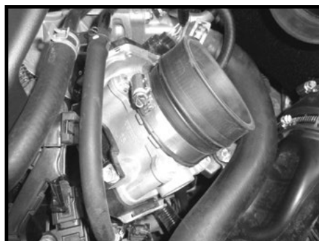
Step 11 Install the 2.75"-3" coupler on the throttle body. Use two clamps, only tighten the one on the throttle body.
