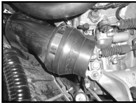
Step 8 Install the 4" to 3" reducer on the fresh air inlet. Use two clamps, only tighten the one on the big side.
