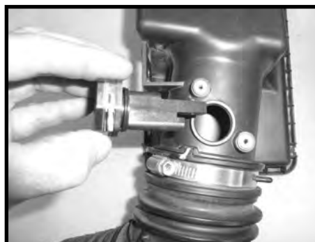
Step 12 Remove the MAF sensor from the stock intake and install it in the aluminum tube.
