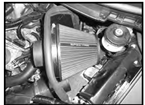
Step 10 Install the air filter on the adapter and clamp in place.
